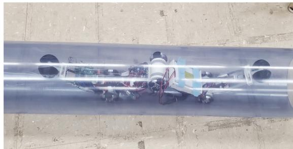
Figure 1. Sensing robot moving in a 6-inch pipe
