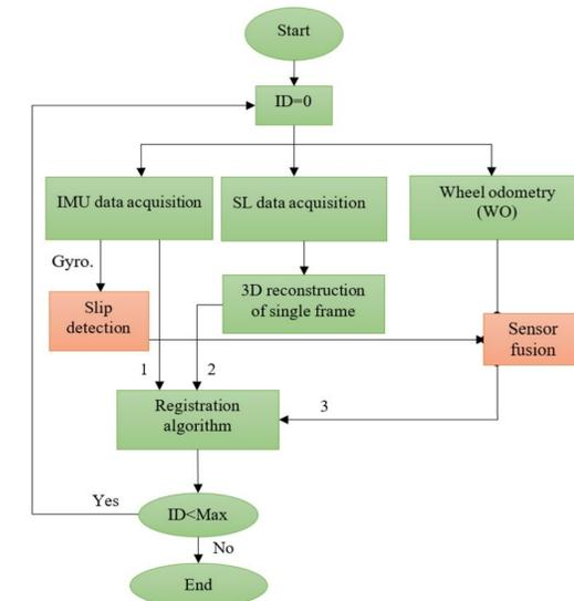
Figure 6. Proposed registration approach for sensor stabilization with data acquisition procedure
