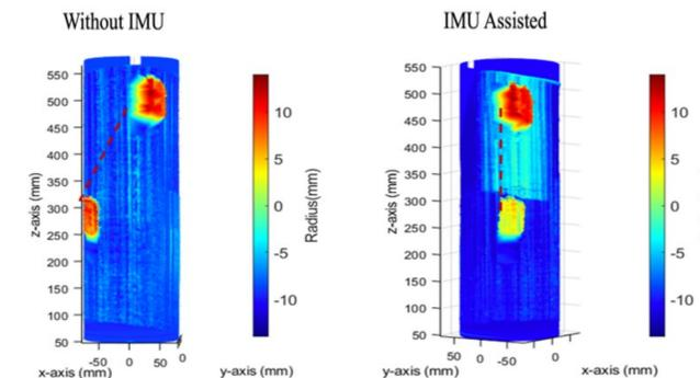
Figure 7. Side view of reconstruction pipe at 25-degree rotation: without IMU (left) and with IMU (right).
