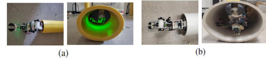
Figure 5. Robotic Sensing system in a) 4inch pipe view b) 6inch pipe view
