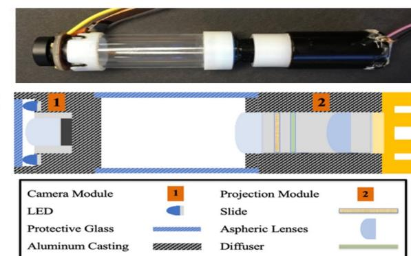
Figure 4. Structured Light Sensor.
