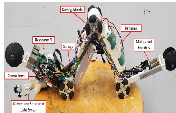
Figure 3. Designed robotic platform.
